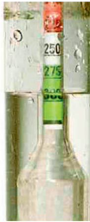
Figure 3.44 Reading a hydrometer: fully charged
